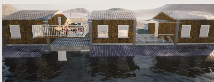
External concrete pillars to existing buildings can allow second stories that can function as vertical evacuation
